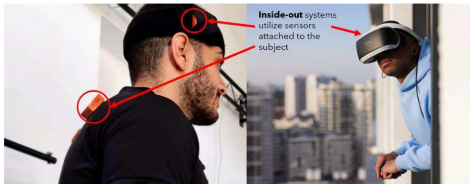
Figure 2.3 Inside-Out systems utilize sensors attached to the subjects to estimate motion 5 .
