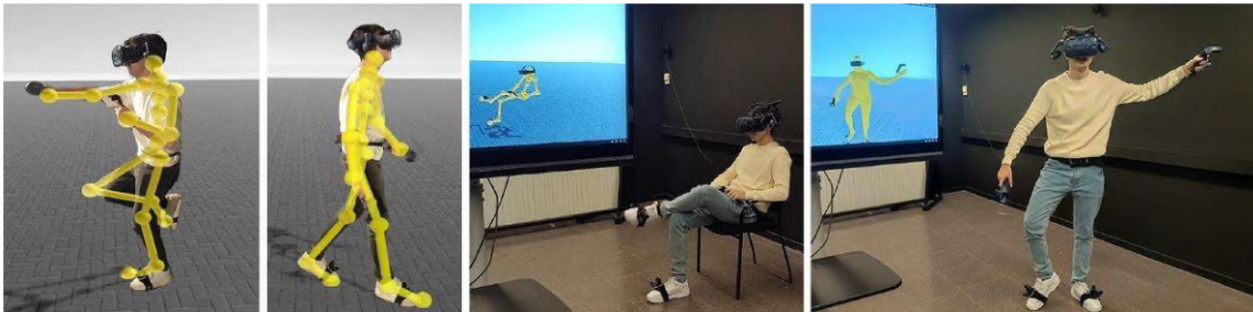
Figure 2: Highly accurate poses reconstructed from six 6-DoF trackers using SparsePoser.
